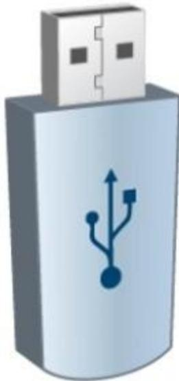
BadUSB tricks the targeted computer into believing that it is not a USB flash drive, but a USB keyboard instead. When you plug in the USB stick, it rapidly sends a string of characters which look to the computer just as though they have been typed at the keyboard by the user.
